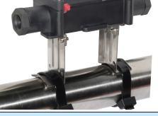
3: One stainless steel bracket, for offset mounting on piping, allowing the enclosure to be locked in after the insulation and its protection have been installed. Allow an insulation thickness of 50 mm, and can be used on hot pipes. Clamping on metal or PVC piping by nylon tie or metal clamp. (Legs available as an accessory.)
