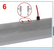
6: If the thermal insulation has a metal protective sheath, make two straight incisions of 4x42mm at a distance of 52mm to allow each of the two legs to pass. Provide the orifice(s) to exit the cables from the metal protection. Equip them with M25 cable glands with the appropriate gaskets for the dimensions of the cables. Close the metal sheath around the tube. Wrap insulation on the pipe, just making two straight cuts for the legs
