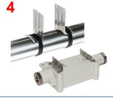
4: Separate the box from the two feet. It will be reassembled after installation of the insulation and any metal protective sheath Assemble on the pipe with cable ties or stainless steel hose clamp
