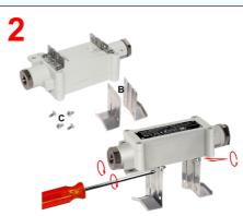
2: Assemble the two feet with the four screws. Take the 2 legs (B) and the 4 screws (C)
